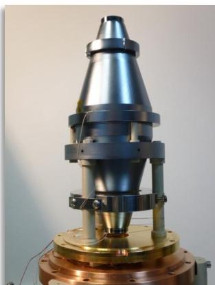
cryogenic 21 cm silicon cavity
