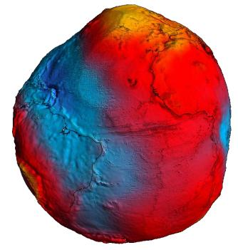
Relativistic geodesy: mapping of the Earth gravitational potential based on the precision measurement of the red-shift experienced by two clocks at two different locations
