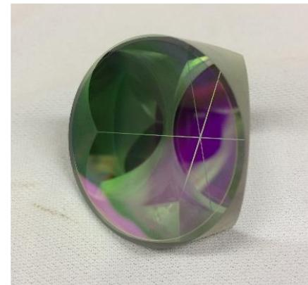
Modified ACES retroreflector with added optical filter layer. Layer is optimized for transmission of 532 nm. Reflector diameter is approx. 38 mm.
