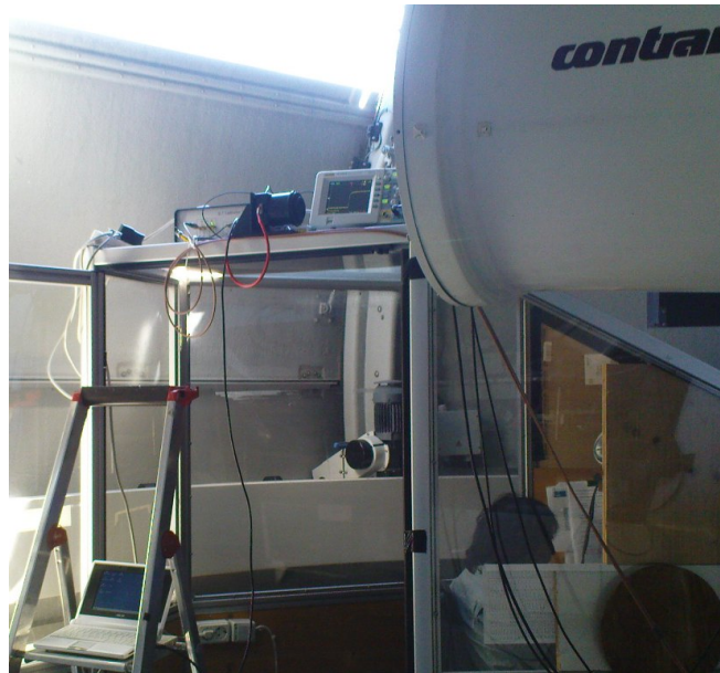
Figure 1 The Calibration Device installed in a dome in front of the Graz SLR system. SLR system telescope (right top), detector (black, top center), Calibration Device Timing unit (top, left), process control and data acquisition PC (low left).
