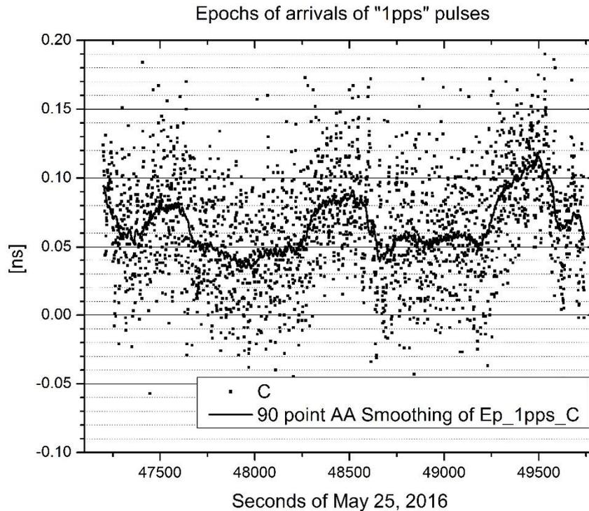
Figure 3a - Plot of fractional epochs of arrival of “1 pps” pulse to the ELT Timing unit input, “standard behavior”. Note the moving average changes reaching  $\pm 50$  ps
