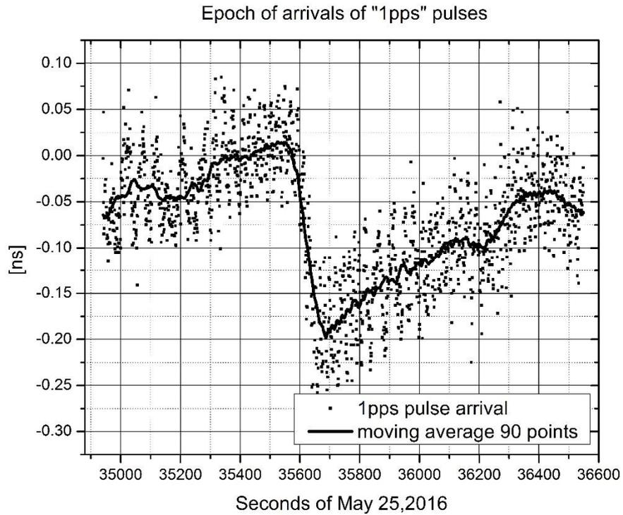
Figure 3b. Plot of fractional epochs of arrival of "1 pps" pulse to the ELT Timing unit input, extreme situation. Note the "jump" exceeding 200 ps.
