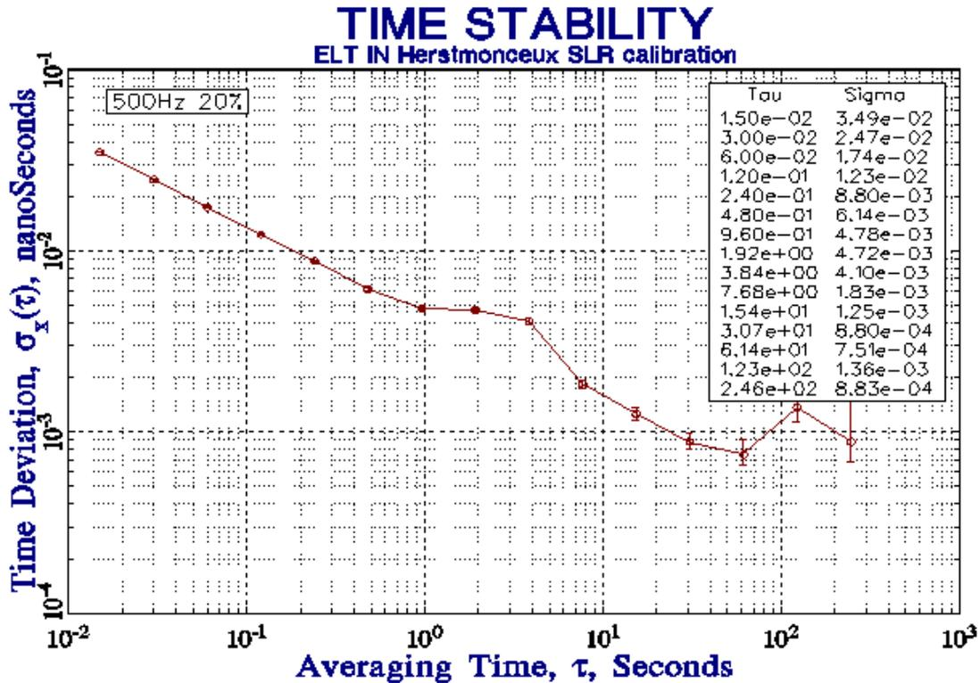
Figure 6 - Overall system performance in a sense of Time deviation TDEV. One can note the value TDEV < 1 ps at 25 to 80 s integration time
