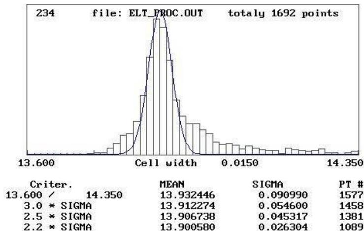
Figure 5 - Histogram of measured epoch (ELT-SLR) differences in series No. 11. All epochs are in ns. Note the measurement jitter of ~26 ps rms.
