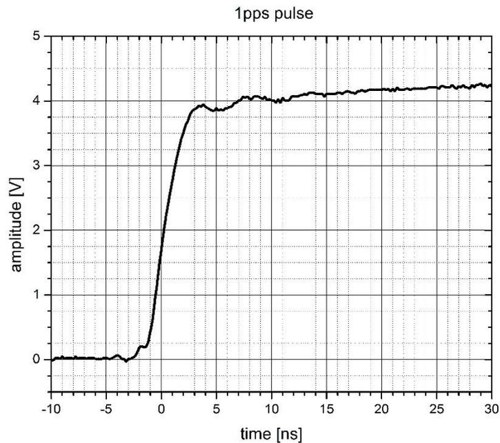
Figure 2 - Time signal "1 pps" on the input of SLR and ELT timing electronics, oscilloscope bandwidth 1 GHz. The trigger level of +1.500 V was used. Signal slew rate ~1 V/ns.
