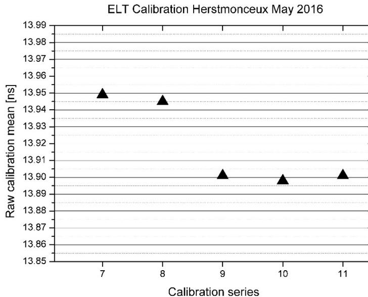
Figure 7 - Raw calibration mean values in series No. 7 to 11.
