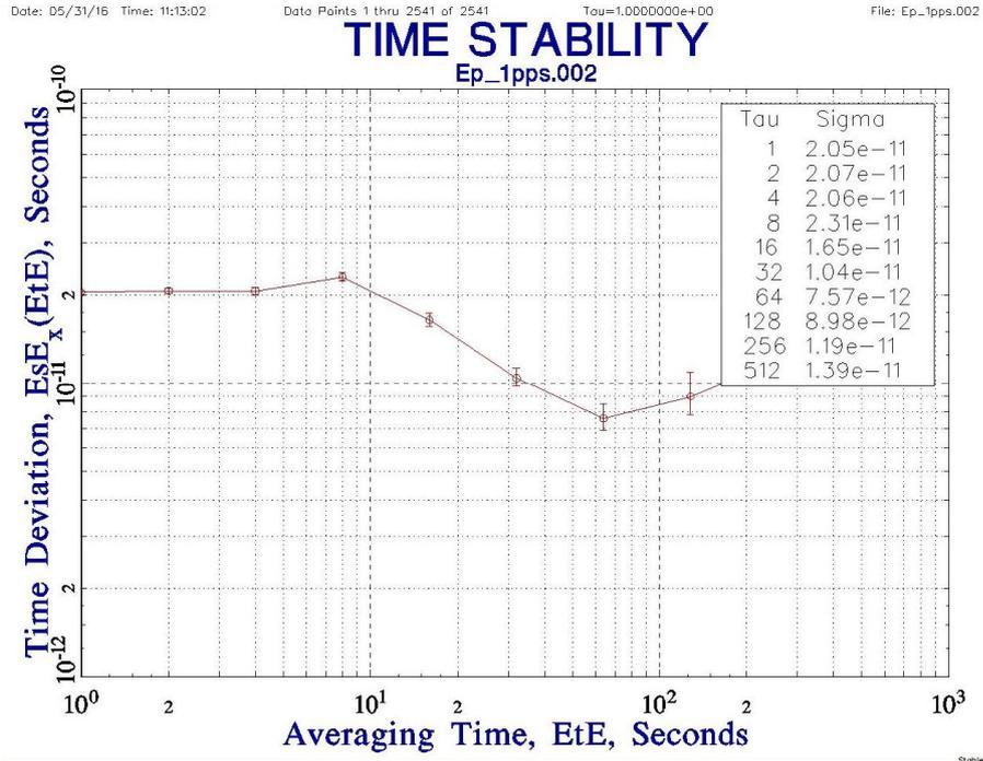
Figure 4 - Timing characteristics of “1 pps” signal expressed as Time Deviation TDEV.
