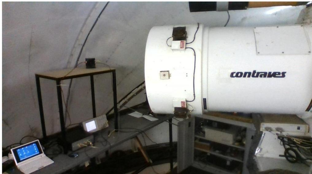
Figure 1 - ELT Calibration Device installed in a dome in front of the Herstmonceux SLR system. SLR system telescope (right top), ELT detector (black, top center), ELT calibration Timing (bottom), process control and data acquisition PC (bottom left).
