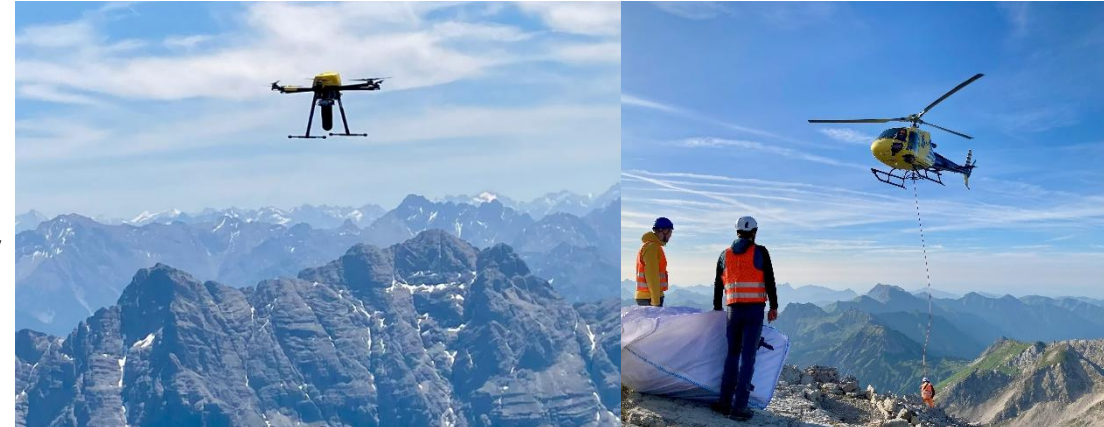
Left: UAV with laser scanner; Right: Measurement campaign at Mt. Hochvogel
