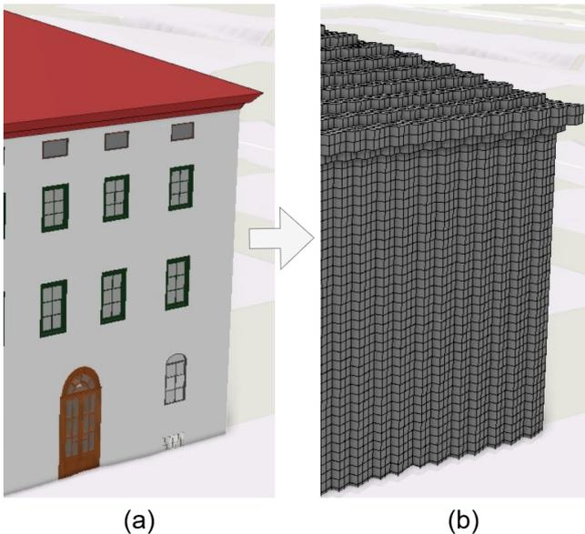
Figure 1: CityGML building model (a) and corresponding voxel representation (b)
