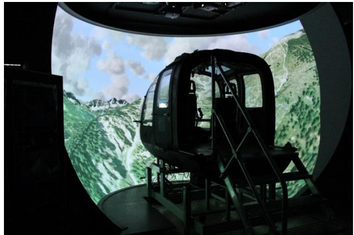
Figure 1: TUM Rotorcraft Simulation Environment
