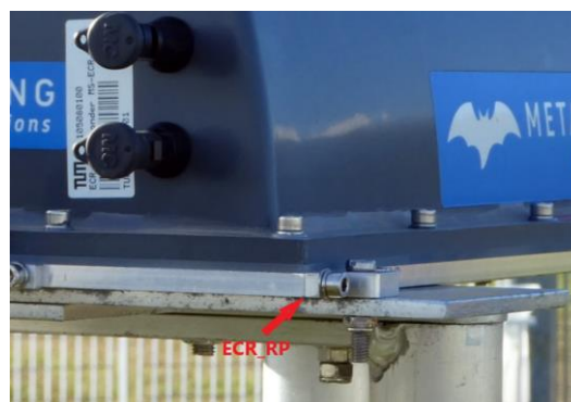
Figure 5-2: Definiton of the ECR Reference Point (RP); Left picture Copyright MetaSensing BV.
