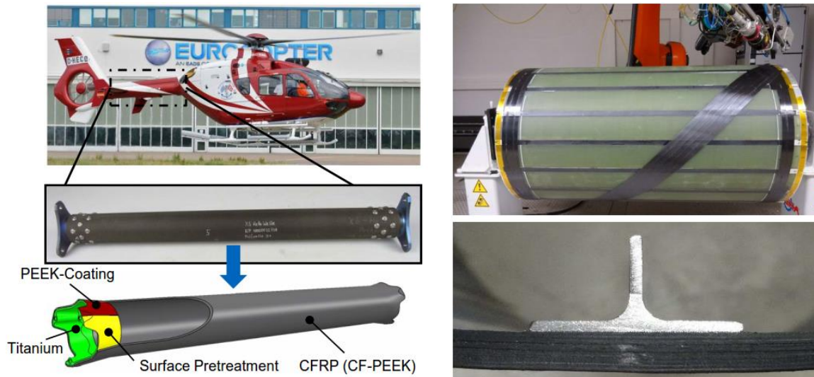
Figure 4. Joints manufactured by AFPisc, left helicopter drive shaft of project TransHybrid, right AL-profile stiffened barrel manufactured in project PolyMet
