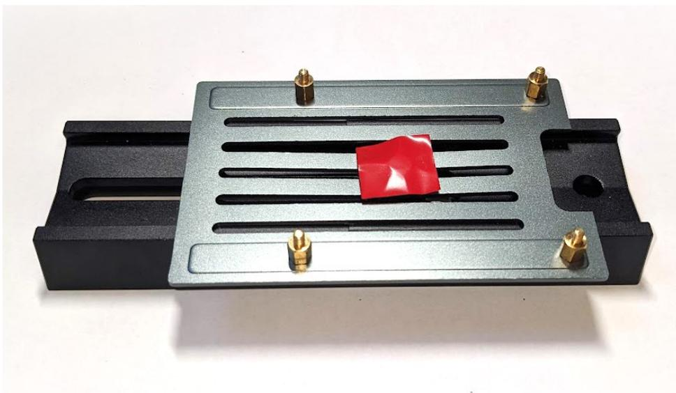
Fig. 2-2: Picture of the assembled bottom plate with covered camera screw and spacer screws attached
