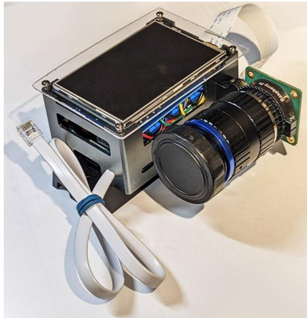
**Fig. 2–9: Picture of the Moon guider with the relay board fully assembled**
