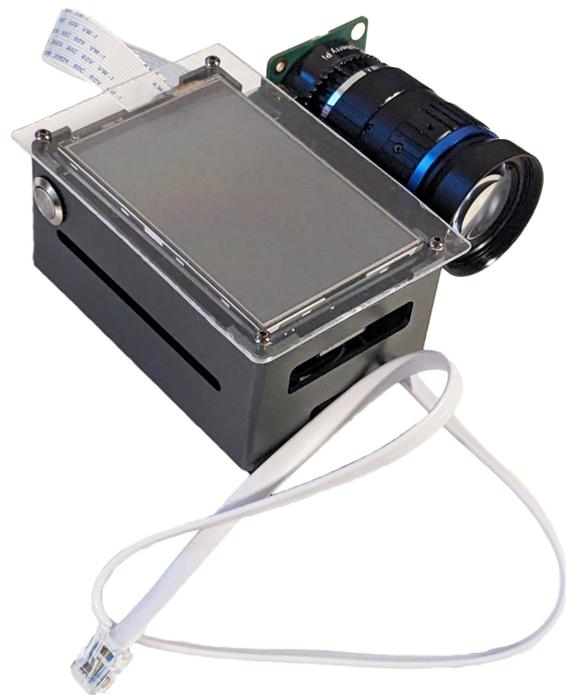
**Fig. 1–1: Picture of the completed Moon guider assembly**
